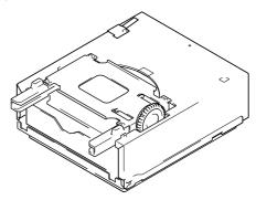
The DRM-UF701 disc flip unit is designed for use in turning over a disc. Note that this component is required when using double-sided DVD discs.
